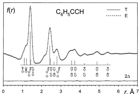
**Figure 6.** Radial distribution curves of ethynylbenzene (E, experimental; T, theoretical). They were calculated using an artificial damping factor  $\exp(-0.002s^2)$ ; theoretical values were used in the  $0.00 \leq s \leq 1.75 \text{ \AA}^{-1}$  region. The positions of the most important distances are marked with vertical bars, whose heights are proportional to the relative weights of the atomic pairs. Also shown is the difference curve ( $E - T$ ).
